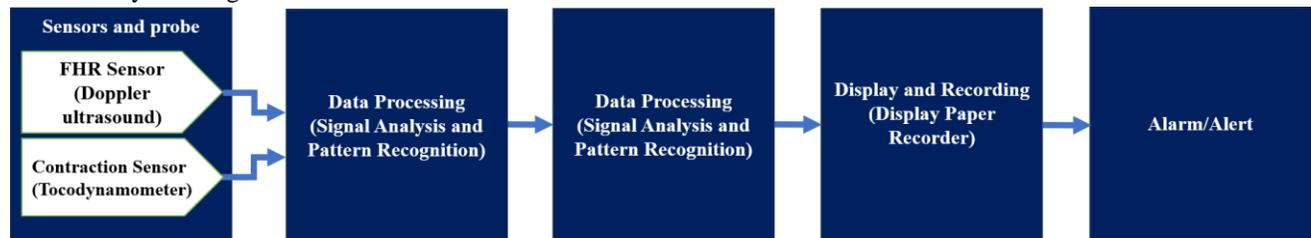
Figure: 2 block diagram of the cardiogram machine.
