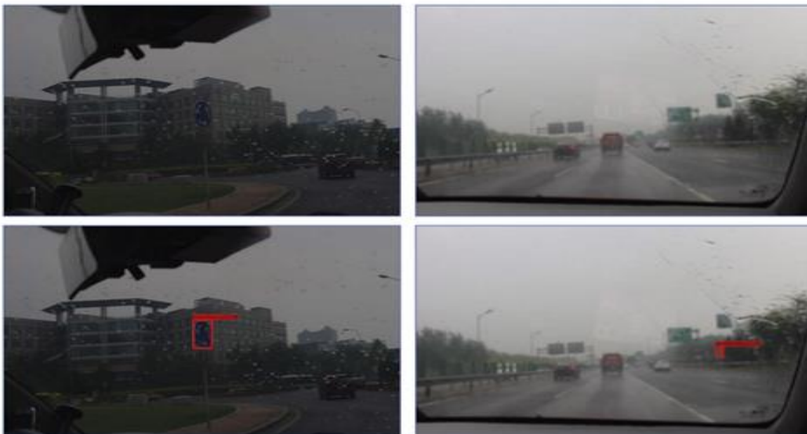
Figure 8: Final detection results by the proposed detection method.
