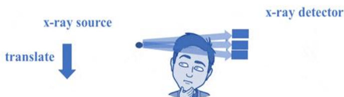
Figure 4: 2nd generation of CT; The translate and rotate acquisition
