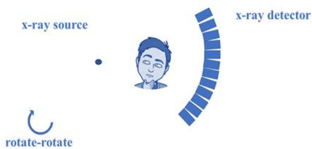
Figure 5: Rotate movement: tube and detector movement of a third generation scanner.
