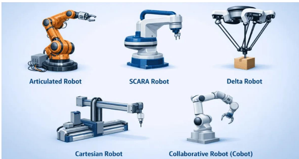
Figure 3: Types of robot arm (Jahanshahi et al., 2024).
