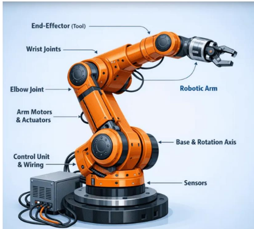
Figure 1: Robot arm description (Joose et al., 2021)
